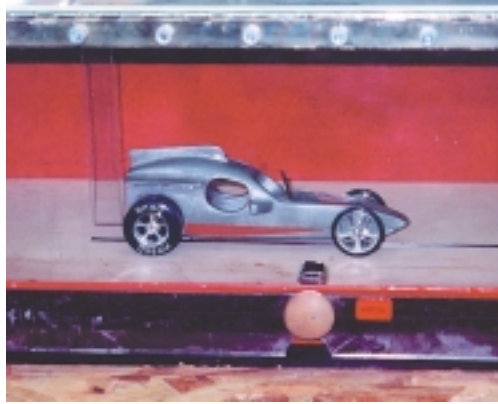
Photo 4—A car in the wind tunnel. Note the lever behind the car, which is attached to the meter.
