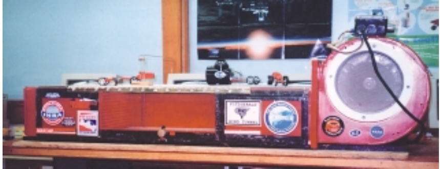
Photo 1—Completed wind tunnel
